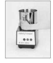
2) Then, turn it back to the right. The magnet bar/handle should come to a stop at the front of the motor base. The bowl, when properly assembled should be just off and level with the top surface of the motor base.
